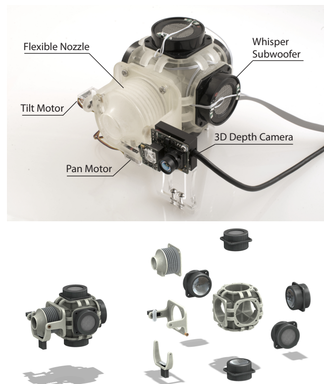
Figure 2: Top: a fully assembled AIREAL device. Bottom: an exploded view showing speakers, the pan and tilt motors as well as the 3D printed enclosure, flexible nozzle and gimbal structures.
