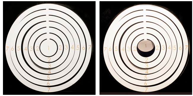
Figure 4: A paper target was used to measure accuracy performance. We show the target at its resting and hit state.
